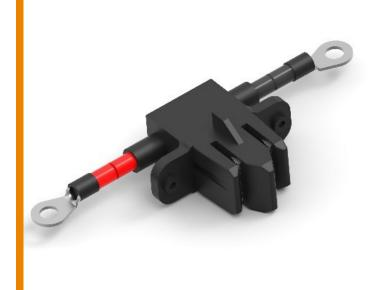
Our new side exit CROWN CLIP Junior cable assemblies enable up to 50% space savings over traditional bus bar cable assemblies. By utilizing a side exit for cables, this solution minimizes the need to bend cables when routing them beyond the center of the server, switch or storage enclosure. These cable assemblies are capable of transmitting power up to 200A.
