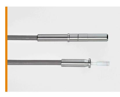
TE Connectivity (TE) has developed its newest rugged expanded beam optical termini — Single Mode (SM) and Multimode (MM) EB16. The EB16 termini are size 16 optical contacts, fit-form compliant with MIL-DTL-38999 Series I and Series III and MIL-STD-1760 lanyard release size 16 AWG cavity.
