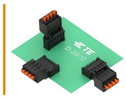
D-2970 Dynamic Series is a compact 5-mm pitch wire-to-board PCB connector with field-installable, time-saving push-in clamp termination.
