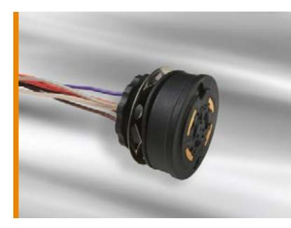
LUMAWISE Endurance N tool-less rotatable dimming receptacle assembly is ANSI C136.41 compliant and hand rotatable up to 355 degrees for outdoor luminaires that require a NEMA based socket. Roadway and street and area lighting applications require an interface between lighting controls and a light fixture that is easily assembled into the light, sealed from harsh outdoor elements and designed for ease of rotation.
